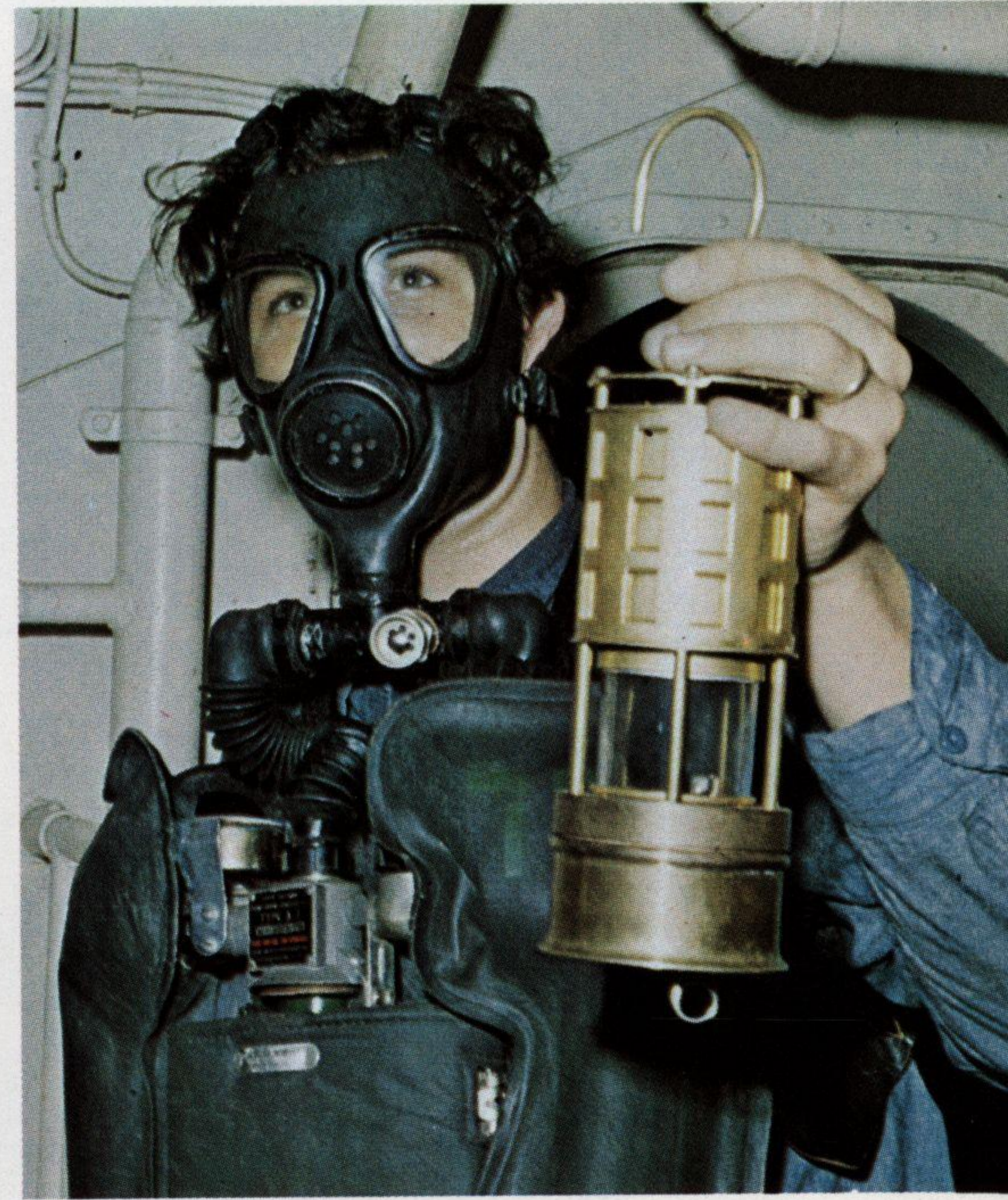
Above Crewman tests for explosive fumes with a flame safety lantern. Left Fire hoses are hooked up to required lengths as each team is called to drill in different spaces.
